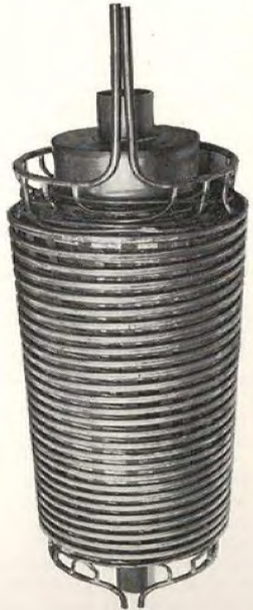
FIGURE 2.24. Three types of heat exchangers used in the NBS hydrogen liquefier.
