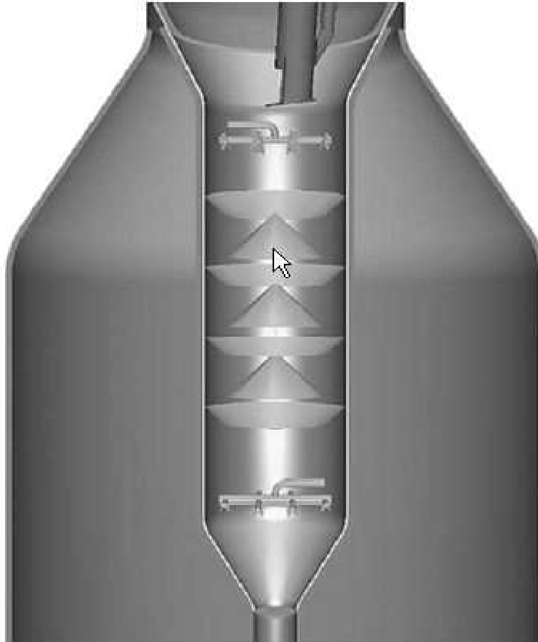
..... Spent catalyst stripper.
