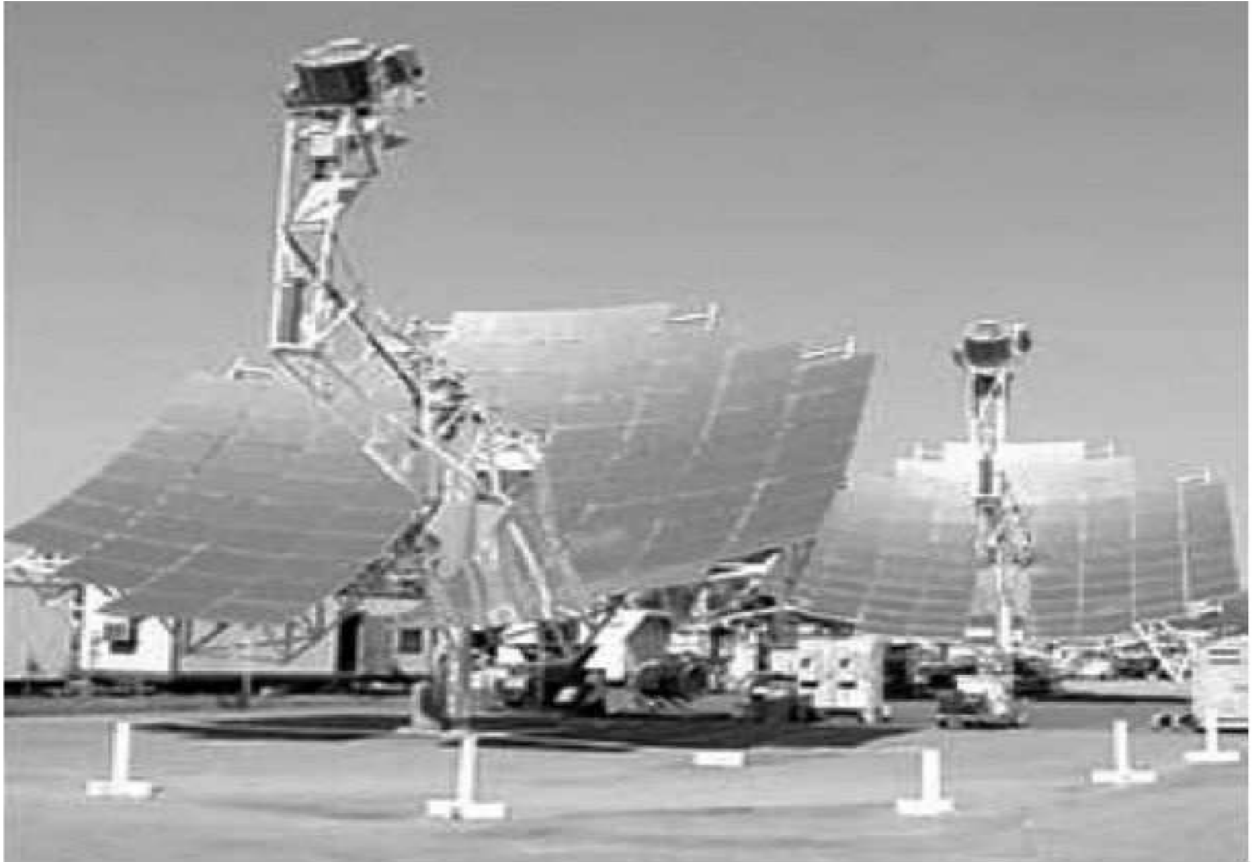
Photograph of a dish concentrator with Stirling engine
